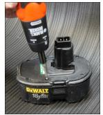
**8**. Once you have a secure fit, you can know tighten down the screws. Over tightening the screws could cause the screws to strip out of there plastic connection.
