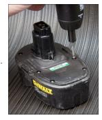
**2.** Take a regular small flat blade screwdriver and place the flat blade tip in to one side of the connection and push down while holding the plastic lid. This may take a little muscle, and be careful when you pull up on the plastic lid.
