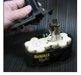
**4.** Turn the bottom case upside down and pull the battery-pack out. If you have trouble getting the battery loose from the case. Take a small hammer and lightly tap the bottom side of the case.
